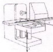
Figure 10.4 Coordinate system for a mill. (Y. Kwon, Computer Control of Manufacturing Systems, McGraw-Hill, 1981)
